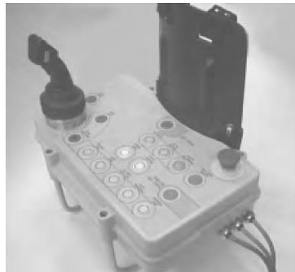
Fig. 6. Remote control (twin bright buttons) with a 6D-joystick.
