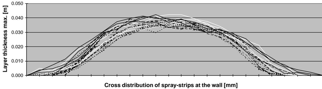
Fig. 11. Concrete cross-distribution curves sprayed in single strips.
