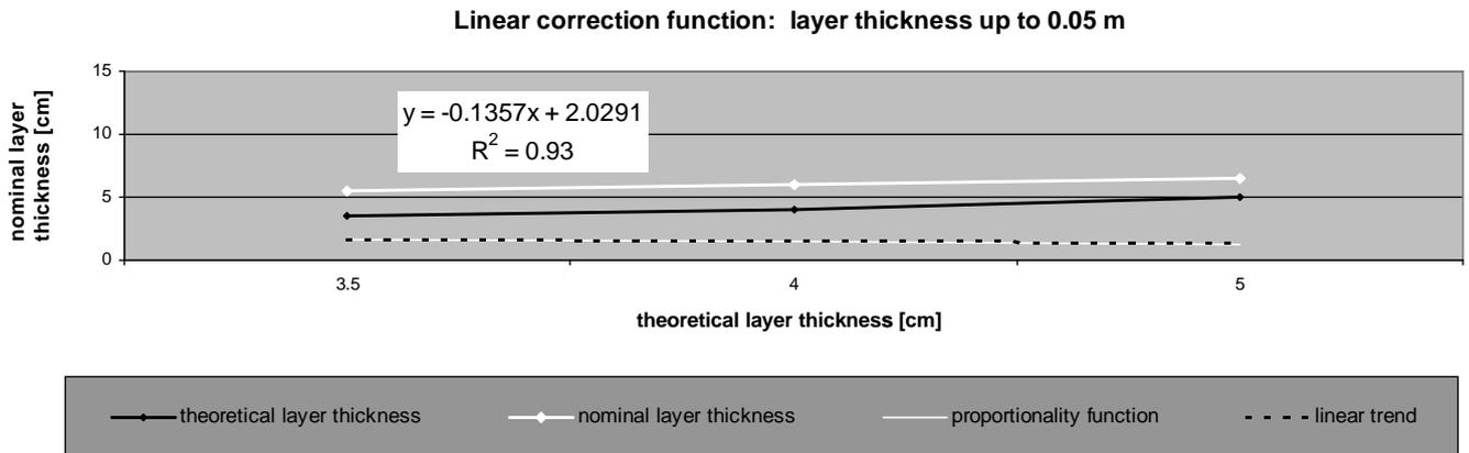
**Fig. 21.** Correction function theoretical-nominal layer thickness (layer thickness up to 0.05 m).
