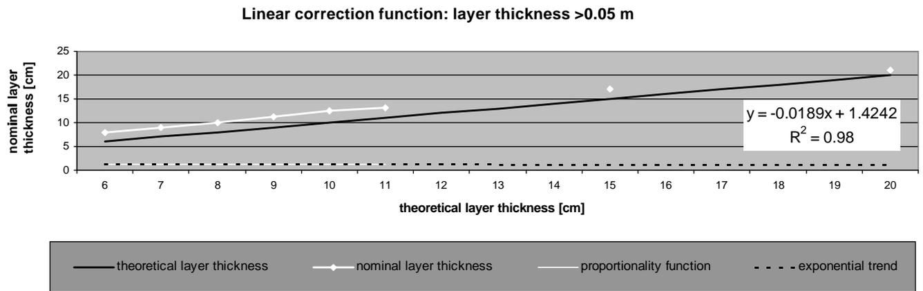
**Fig. 22.** Correction function theoretical-nominal layer thickness (layer thickness > 0.05 m).
