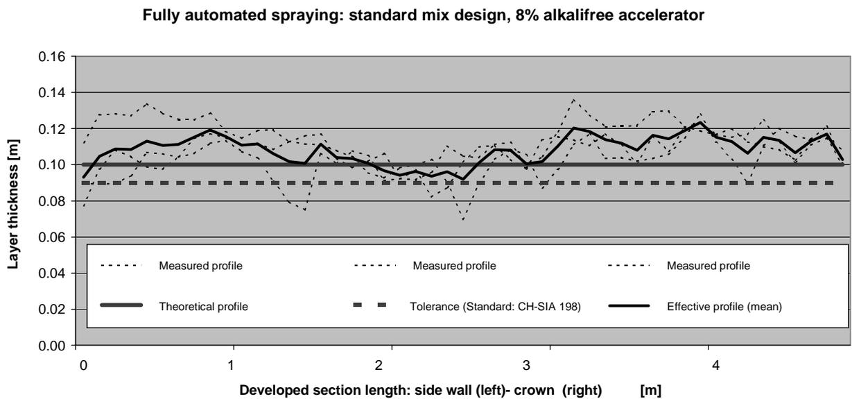
**Fig. 23.** Layer control of fully automated shotcrete application.
