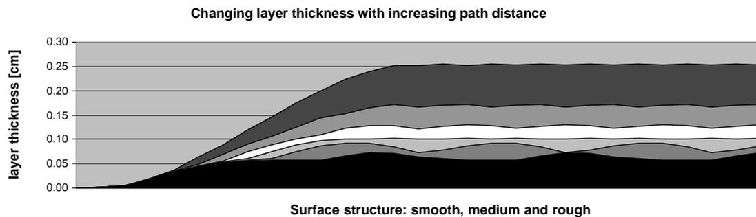
Fig. 16. Evenness of different final layer thicknesses.
