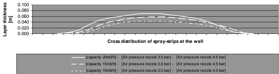
Fig. 19. Increase of design profiles from 0.04 up to 0.07 m with enlarged concrete capacity ( $R_{nozzle} = 2 \text{ rps}$ ).
