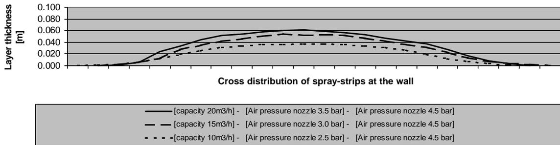
Fig. 18. Increase of design profiles from 0.04 up to 0.06 m with enlarged concrete capacity ( $R_{nozzle} = 1 \text{ rps}$ ).
